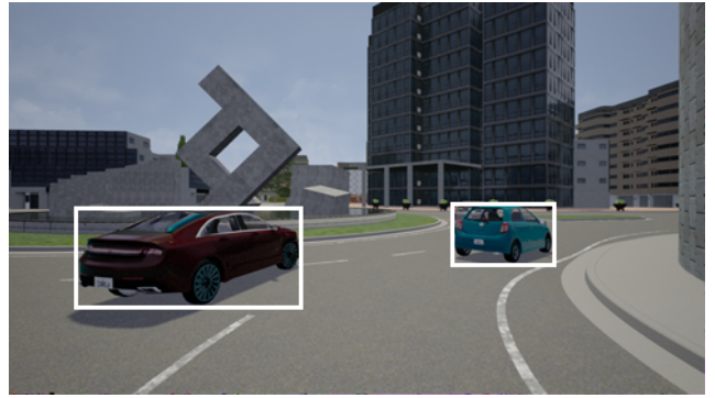
(b) Given an RGB image, the detector outputs a bounding box for each detected object. In this example, a vehicle on the right occludes another, so only two objects are detected. As the detector has no knowledge of the mapping from bounding boxes to vehicles, detected bounding boxes are shown as solid white rectangles, rather than colored based on the targets being tracked, as in inset (a).
