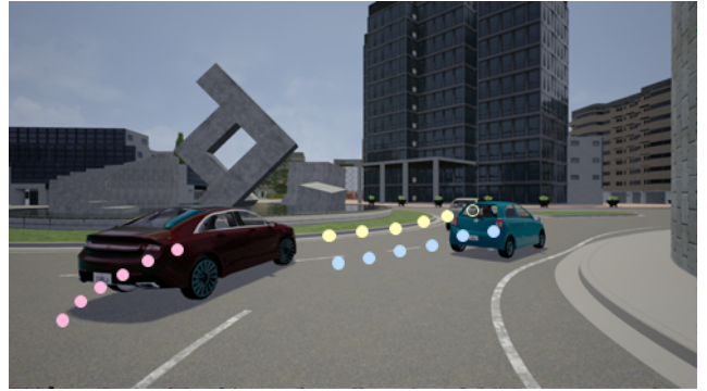
(d) Tracks matched to a detection are updated with a new position based on that detection. Unmatched tracks are either deleted (if unmatched long enough) or updated with the predicted position.
