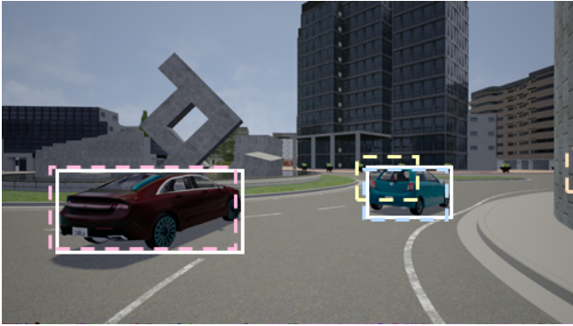
(c) Matching occurs between the predicted positions of each track and the detected bounding boxes. In this example, two of the four tracks are matched to a detection.
