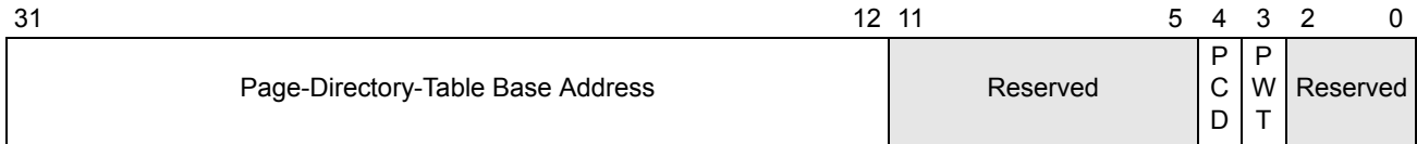
Figure 3-4. Control Register 3 (CR3)—Legacy-Mode Non-PAE Paging
