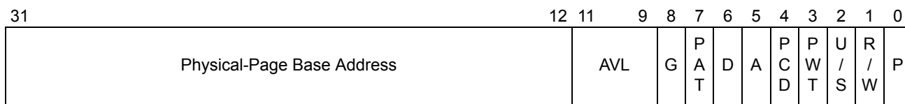
Figure 5-6. 4-Kbyte PTE—Non-PAE Paging Legacy-Mode
