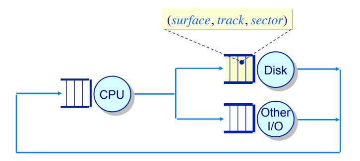
The OS maximizes disk I/O throughput by minimizing head movement through disk head scheduling
