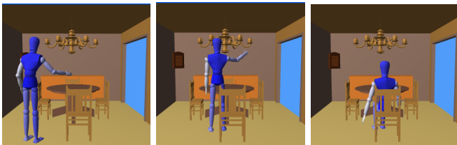
Fig. 8. The robot moves toward one chair and sits down. To avoid the collision with the overhead light, the robot needs to bend itself. This scenario has narrow passages and tight spaces, and therefore, the planner takes more time.
