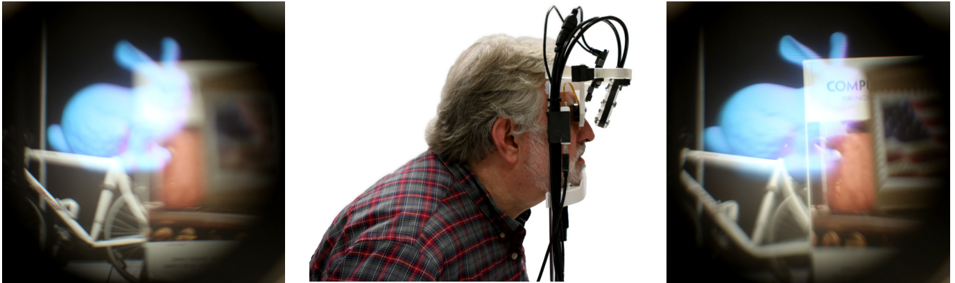
Fig. 1. Left: The view of both real and virtual for a presbyopic user with distant vision, with the accommodation depth fixed at 7 m, on a conventional AR HMD. The virtual bunny is at a mid-distance (1 m) together with the stamp (0.25 m), text book (1 m) and bicycle (5 m) arranged at near, medium and far distances respectively. Notice that both the real and virtual imagery appears blurred to the user as none of the objects are in the presbyopic user's accommodation plane. Middle: A presbyopic user with near zero accommodation range looking through our auto-focus AR eyeglasses. Our prototype AR eyeglasses are capable of providing well-focused imagery of both real and virtual objects at all depths by independently adjusting for the user focus for viewing both real world and virtual imagery from the internal display, based on the user's current eye accommodation state. Right: The well-focused view of both real and virtual objects of the same scene on our auto-focus AR eyeglasses, due to independent focus adjustments for both real and virtual. Notice that the letters on the textbook at the mid-distance (1 m) are in sharp focus, as well as the virtual bunny, which also is set to appear at the mid-distance.
