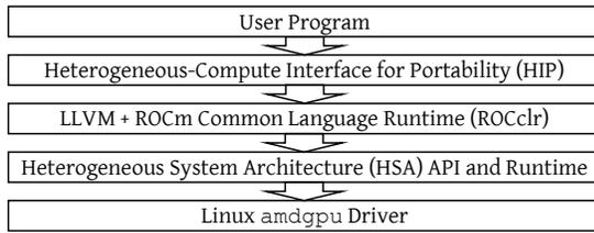
**Figure 2: Components of the ROCm software stack.**
