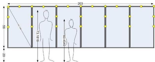
A 6-panel display telepresence wall design, showing the participant scale.
