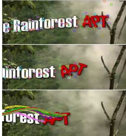
Figure 5: (Top): Initial optical flow. (Middle): salient points with short trajectories in background are discarded. (Lower): Trajectories on non-codeword characters are also discarded.
