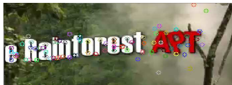
Figure 4: The circles depict salient features. These salient features are usually corners of an object or texture areas.
