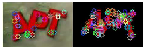
Figure 7: re-running tracking with a lower threshold on corner quality: Left: before modification. Right: after modification.
