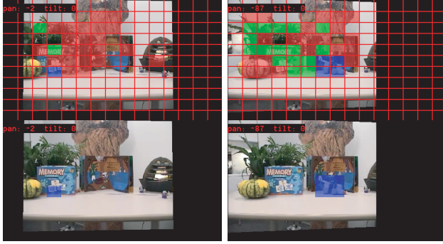
Figure 3. Indoor Sequence. Top row: Color-coded output of the detection procedures associated to the models M_1 , M_2 , and M_3 . See Figure 2 for color descriptions. Bottom row: salient motion detection results. The images on the left contain some false alarms, which could easily be removed by a temporal filter.
