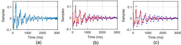
Figure 9: Predicting missing values of signal(a) using linear(b) and spline(c) interpolation.
