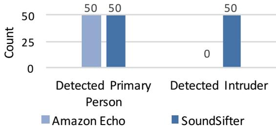
Figure 21: For personalized mode, SoundSifter was able to detect all 50 intruder’s commands, Amazon Echo fails to detect any of them.
