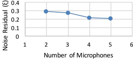
Figure 4: Source separation error for different number of microphones.
