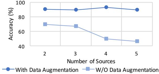
Figure 17: SoundSifter’s data augmentation technique improves modeling accuracy
