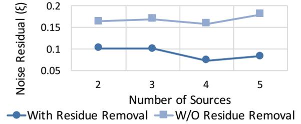
Figure 19: Residue Removal reduces noise residual from the primary signal.
