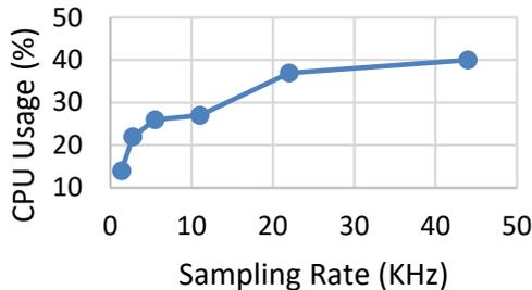
Figure 5: CPU usage increases with sampling rate.
