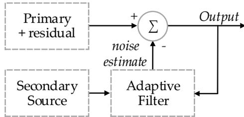
Figure 10: Leveraging isolated secondary sources to nullify their residue through a customized adaptive noise cancellation process.
