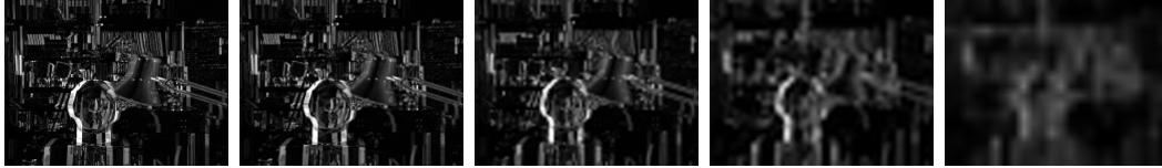
Fig. 5. A single AD image at different mipmap levels, from zero to four, corresponding to a support kernel from 1 \times 1 to 16 \times 16 .
