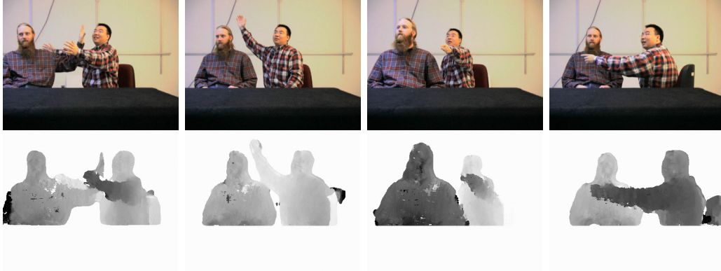
Fig. 14. Stereo (two-camera) results from the live system. The first column shows the input images; the second column shows the disparity map.
