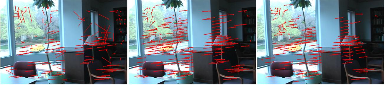
Figure 5. Feature Tracking using (First) Local-adaptive KLT (Second) Our method with known response (Third) Our method with unknown response. The video can be seen at <http://www.cs.unc.edu/~sjkim/klt/tracks.wmv>
