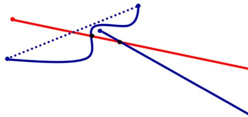
**Figure 1:** With double precision segments defined by endpoints, we cannot test the precise location of an intersection, much less sort intersection points by  $x$ -coordinate. The restricted precision means that we may as well think of segments as curvy “spaghetti.”
