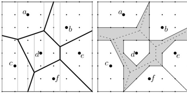
**Figure 2:** *Left:* The trapezoidation, in grey, of a Voronoi diagram, in black, of five sites. *Right:* The Voronoi Polygon Set, shown as white polygons, is a double precision representation of the grid points in each Voronoi cell. To recover the Voronoi diagram's precise structure in the grey gaps requires more than double precision.
