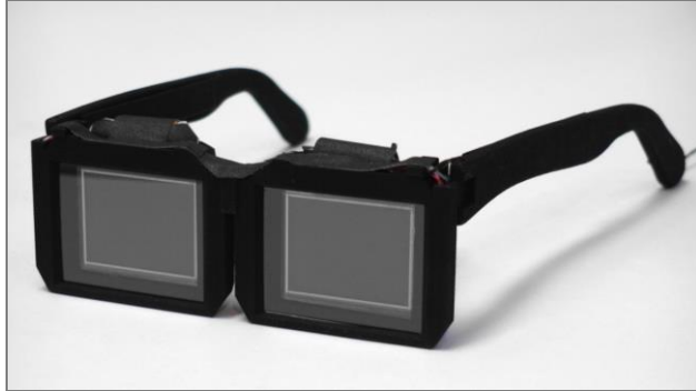
Figure 1: Prototype glasses offering a field of view of 100° diagonal in a package resembling eyeglasses.
