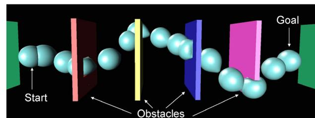
**Figure 2:** Planning results for a deforming sphere navigating through a series of walls. The sphere has over 5,000 surface elements.
