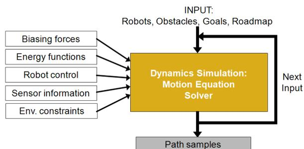
**Figure 1:** Physically-based Motion Planning system architecture. Inputs including artificial biasing forces, the environment, and the agent state are used to generate the next configuration for the agent.
