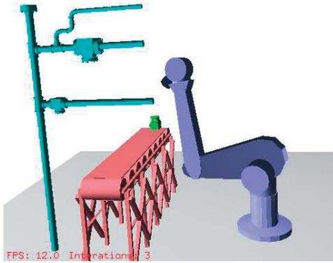
The robot arm must access a part on the moving conveyor belt, while avoiding a piping structure. The moving obstruction causes the robot to reactively modify its path to avoid collision.
