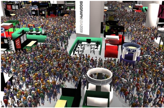
Simulation of a large trade show floor. 80,000 people are simulated at 800 ms/frame on a desktop PC.
