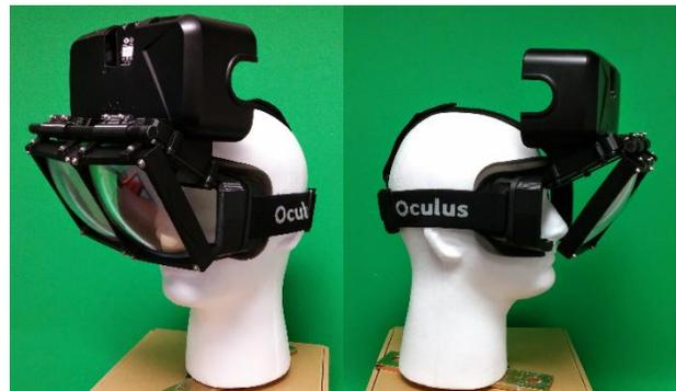
Final design incorporating the curved beam-splitter lenses with screen and tracking sensors from Rift DK2.
