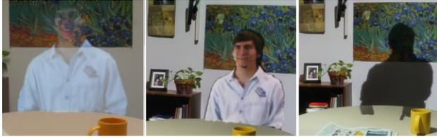
Figure 3: Left: Augmented participant using see-through display appears semi-transparent and ghostly. Center: Augmented participant using projector based lighting appears solid and opaque. Right: Controlled lighting in area of scene behind remote participant.
