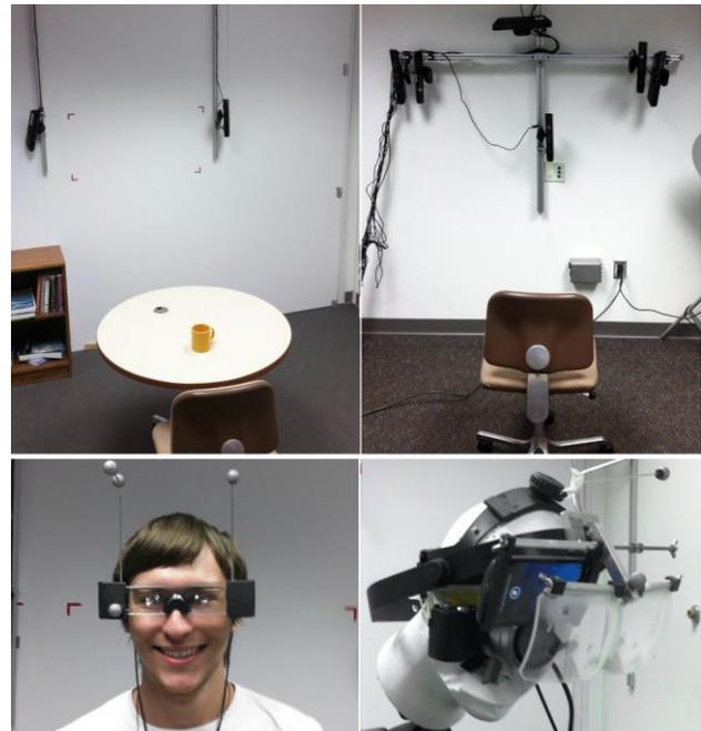
Figure 2: Top row: depth sensor scanning arrays at local and remote sites. Bottom row: commercial and experimental wide field of view displays used to display augmented imagery.
